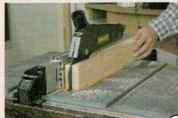
(Above) A roller stand is used for longer work, although a take-off table is better. (Right top) A two position fence can be used for ripping thin material safely (above) and ripping deep timber (below)
