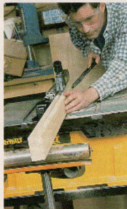
(Above) A roller stand is used for longer work, although a take-off table is better. (Right top) A two position fence can be used for ripping thin material safely (above) and ripping deep timber (below)
